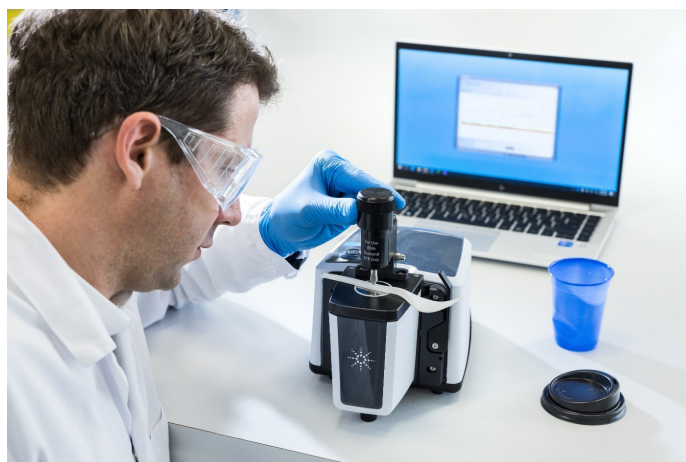
Figure 6. The Agilent Cary 630 FTIR spectrometer can help to identify the source of larger sized pieces of plastic.
