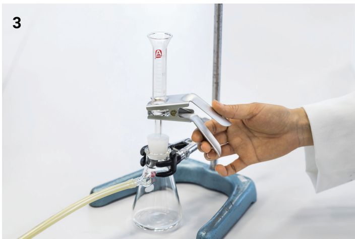
Figure 3. Sample filtration equipment and steps for the preparation of samples for LDIR on-filter analysis.
