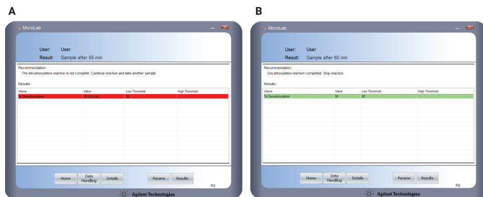
Figure 6. The DELIC Labs-developed decarboxylation model is used within Agilent MicroLab Software. After data acquisition, the software directly reports the percent decarboxylation of the sample. Color-coding facilitates results interpretation and subsequent decision making, while result dependent recommendations help the operator optimize the decarboxylation process.
