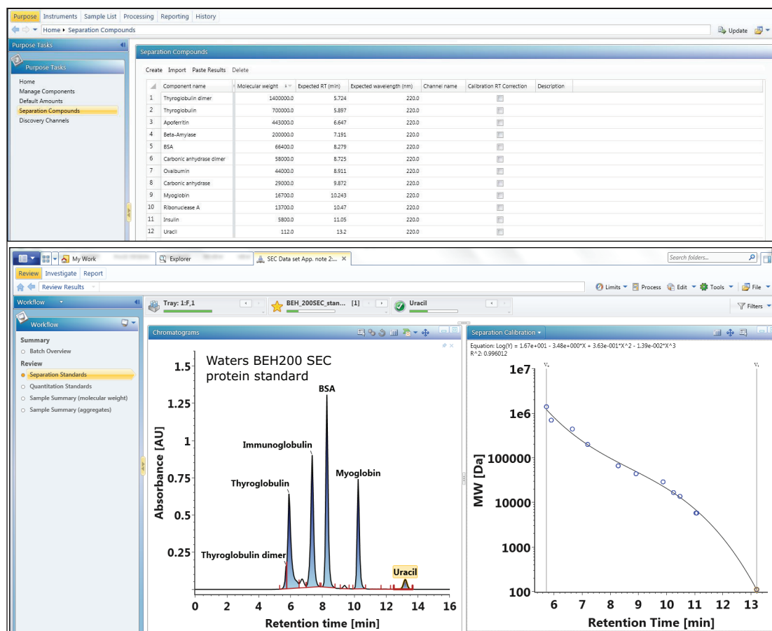
Figure 1. Waters BEH200 SEC protein standards (p/n 186006518) are separated (bottom left panel) using an ACQUITY UPLC Protein BEH SEC Column (p/n186005225). A separation calibration plot of log MW versus retention time (lower right panel) is automatically constructed using UNIFI informatics tools from a set of defined protein standards (top panel).
