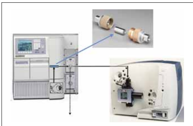
Figure 2. LC/ESI-TOF MS configuration. A Waters Alliance HPLC 2796 Bioseparations System was directly coupled to a Waters LCT Premier ESI-TOF MS for antibody mass analysis. A modern configuration would use the Waters ACQUITY UPLC H-Class Bio System with a Waters Xevo® G2 ToF Mass Spectrometer.
