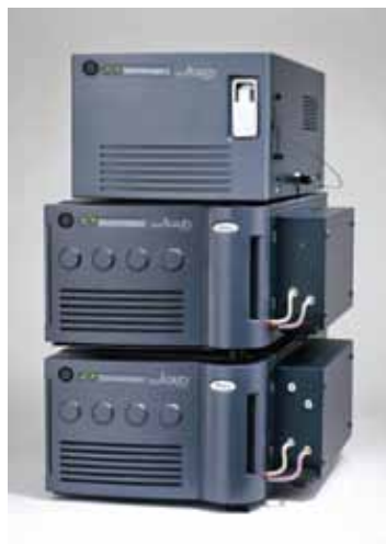
Figure 1. nanoACQUITY UPLC System with HDX Technology. HDX Manager, Binary Solvent Manager (BSM), and Auxiliary Solvent Manager (ASM) are shown from top to bottom, respectively. The HDX Manager is a key component, which can perform the online pepsin digestion and maintain the low temperature at 0 °C required for HDX MS.
