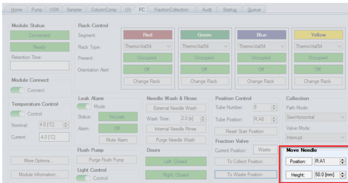
Figure 9. Collection needle height positioning can be customized for flexible positioning of needle. For example, against the liquid level in InVial mode or against sample container height in AboveVial mode.
