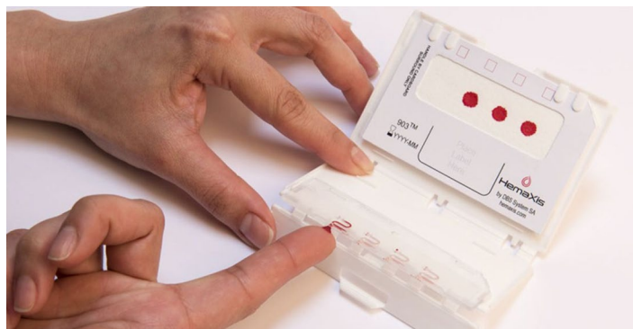
Figure 1. HemaXis DB10 blood collection device precisely collects 10 \mu L blood via capillary action.
