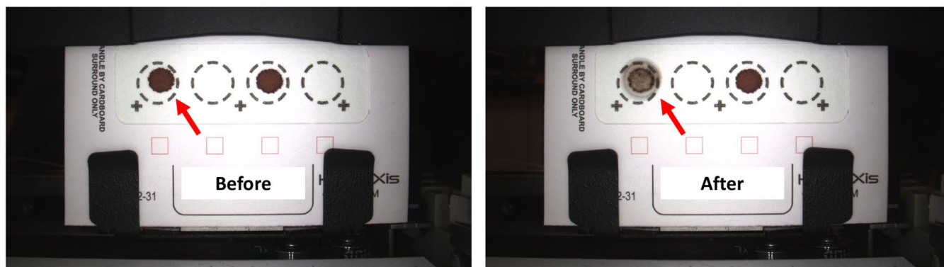
Figure 3. Images of 10 \mu L dried blood spots collected by the HemaXis DB10 device before and after extraction. The Intelligent Vision Camera (IVC) recognizes the actual location of the blood spot and positions the sample spot to the center of the extraction clamp.
