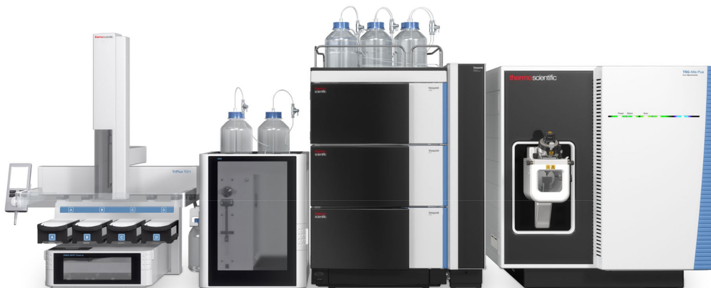
Figure 2. Transcend DSX-1 system and TSQ Altis Plus triple quadrupole mass spectrometer
