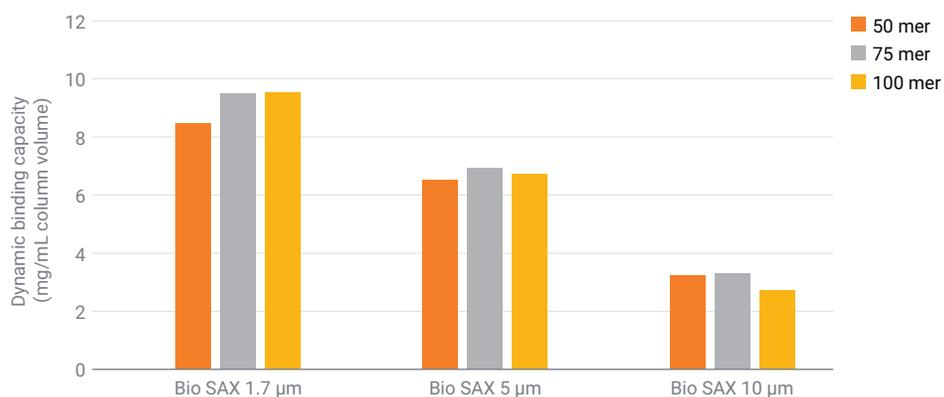
**Figure 2.** Comparison of binding capacity of different size oligonucleotides.
