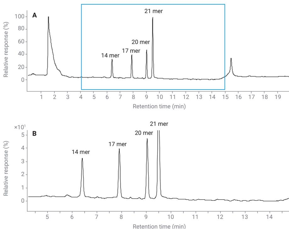
**Figure 4.** Analytical separation of RNA standards using an Agilent Bio SAX 5  $\mu$ m column (A) with zoomed region (B).
