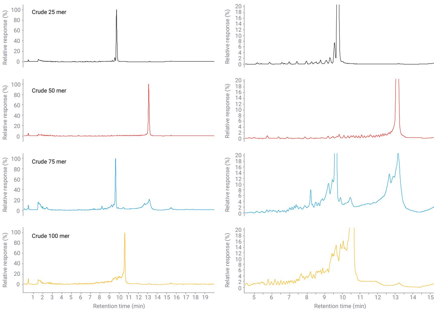
**Figure 3.** Analytical separation of crude 25, 50, 75, and 100 mer using an Agilent Bio SAX 5  $\mu\text{m}$  column (left) with zoomed regions (right).
