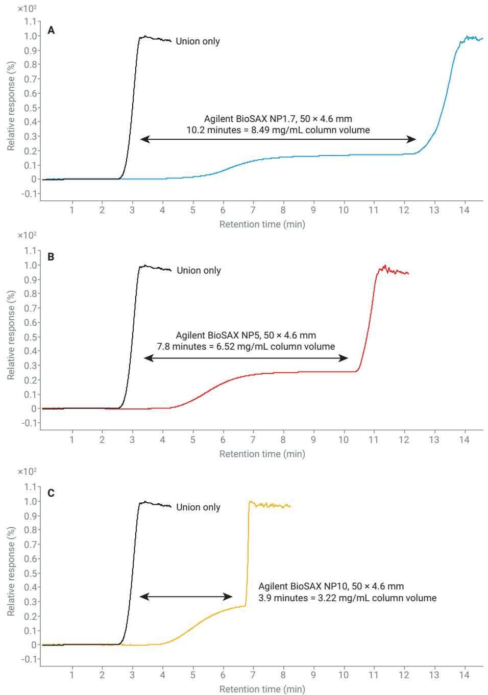
**Figure 1.** 50 mer oligonucleotide breakthroughs using Agilent Bio SAX columns of different sizes: (A) 1.7  $\mu\text{m}$ , (B) 5  $\mu\text{m}$ , and (C) 10  $\mu\text{m}$ .
