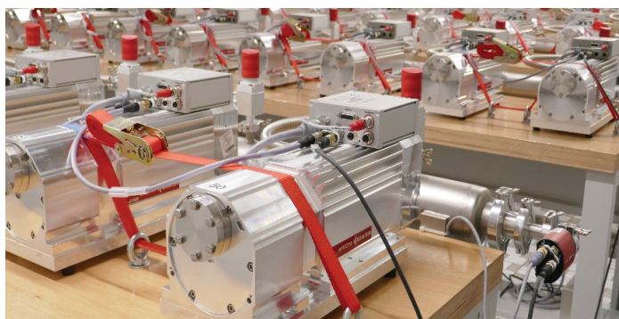
Figure 1. The turbo pumps used in the Orbitrap Exploris 480 mass spectrometer system were tested extensively for long-term performance.
