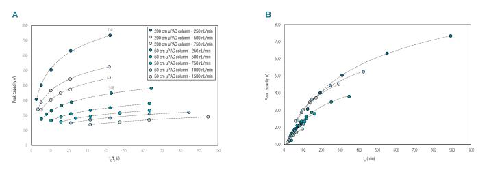
Figure 3. FWHM based peak capacity obtained for an oligonucleotide reference standard mixture (T5-T30). The performance obtained on a 200 cm and a 50 cm  $\mu$ PAC column is compared at different flow rates (250–1500 nL/min). A) Peak capacity plotted as a function of  $t_e/t_o$ .  $t_e=t_n-t_n$ . B) Peak capacity plotted as a function of  $t_n$ , retention time of the last eluting oligonucleotide (T30).
