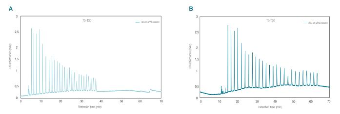
Figure 2. UV chromatograms obtained for the separation of 5-30mer deoxythymidines (dTs) on either A) the 50 cm μPAC column or B) 200 cm μPAC column. Flow rate 750 nL/min, 60 min gradient 20 to 70%B\_C2 curve, A: 100% H<sub>2</sub>O, B: 40% MeOH, UV 260 nm.
