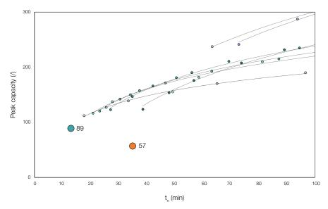
Figure 10. FWHM based peak capacity obtained for a 5mer deoxythymidine oligonucleotide with 4 phosphorothioate linkages (T5-1-4S) on either a 50 cm  $\mu$ PAC column and 15 cm packed bed A column. Peak capacity within the diastereomer elution window is calculated based on the peak width of a baseline separated peak and plotted as a function of t<sub>n</sub>, retention time of the last eluting oligonucleotide diastereomer. Data points have been obtained from separations shown in Figure 9.
