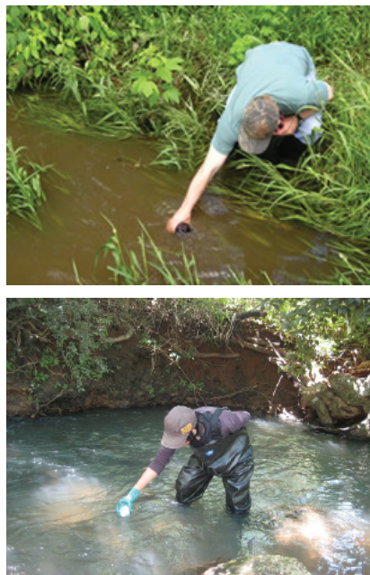
Figure 2: Direct method surface water sampling collection technique
