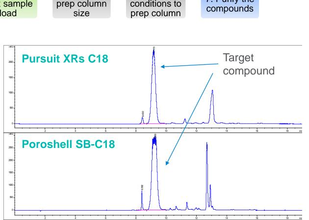
Flow rate: XRs C18 - 1 mL/min; SB-C18 - 0.5 mL/min; mobile phase: A - water + 0.1% formic acid; B - acetonitrile + 0.1% formic acid; gradient: 5 - 95% B in 15 min, 95% B for 3 min; injection volume: XRs C18 - 20 µL; SB-C18 - 10 µL; detection: UV 335 nm.
