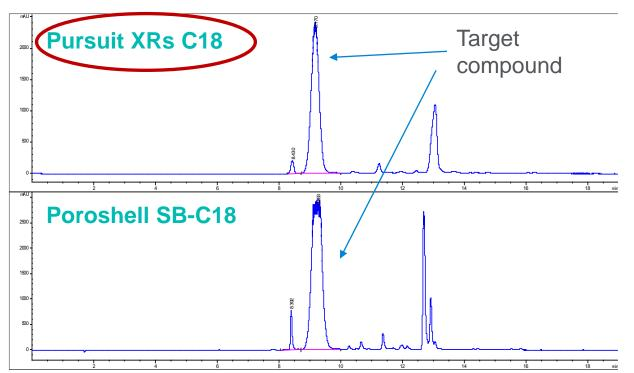
Flow rate: XRs C18 – 1 mL/min; SB-C18 – 0.5 mL/min; mobile phase: A – water + 0.1% formic acid; B – acetonitrile + 0.1% formic acid; gradient: 5 – 95% B in 15 min, 95% B for 3 min; injection volume: XRs C18 – 20 μL; SB-C18 – 10 μL; detection: UV 335 nm.
