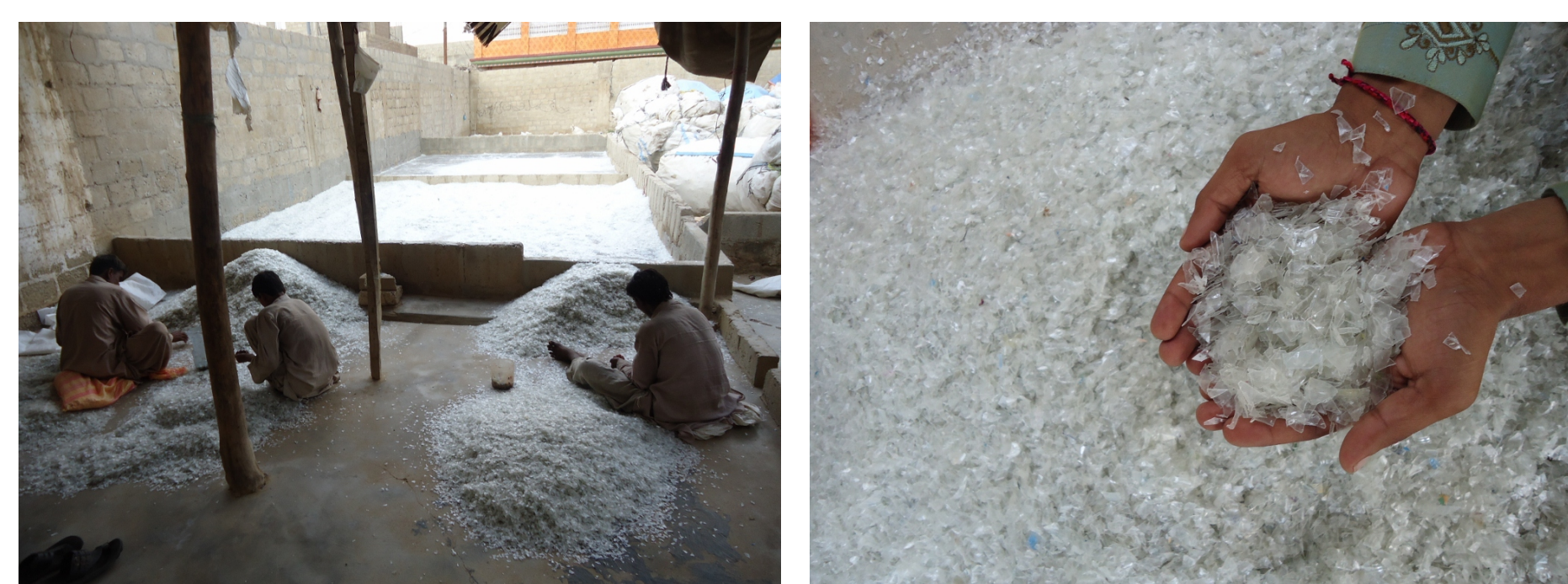
Figure 3 and 4: Sorting of grinded PET bottles on impurities in Pakistan.
