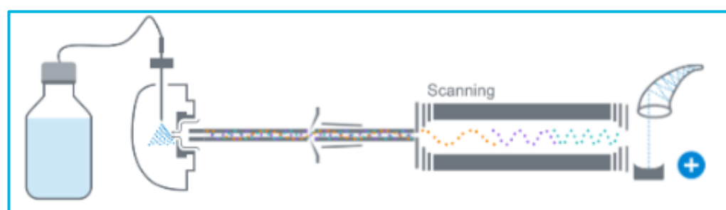
Figure 2. Schematic of LC/SQ mass spectrometer
