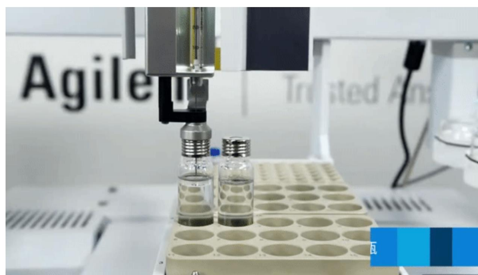
Figure 3. Left: automated vortex at 2000 r/m; Right: transfer 200 \mu L supernatant automatically.
