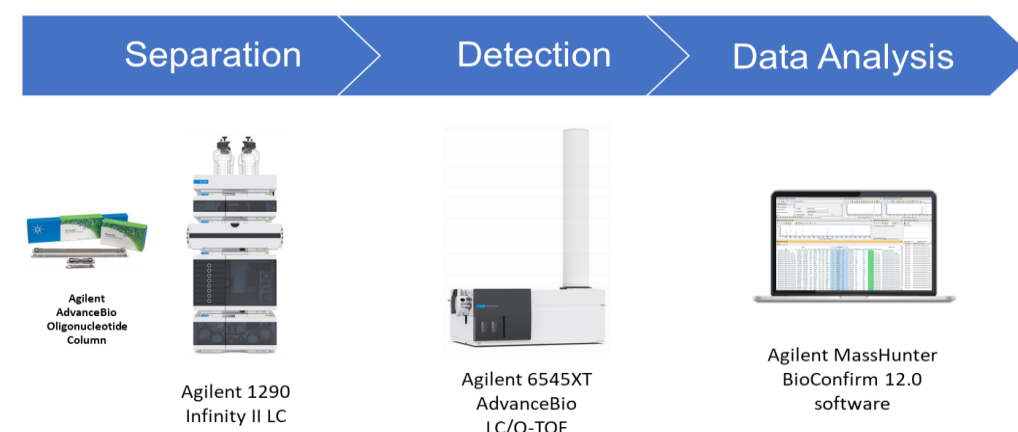
Figure 3. Analytical components of the oligonucleotide analysis - Target Plus Impurities (TPI) and Sequence Confirmation workflows.
