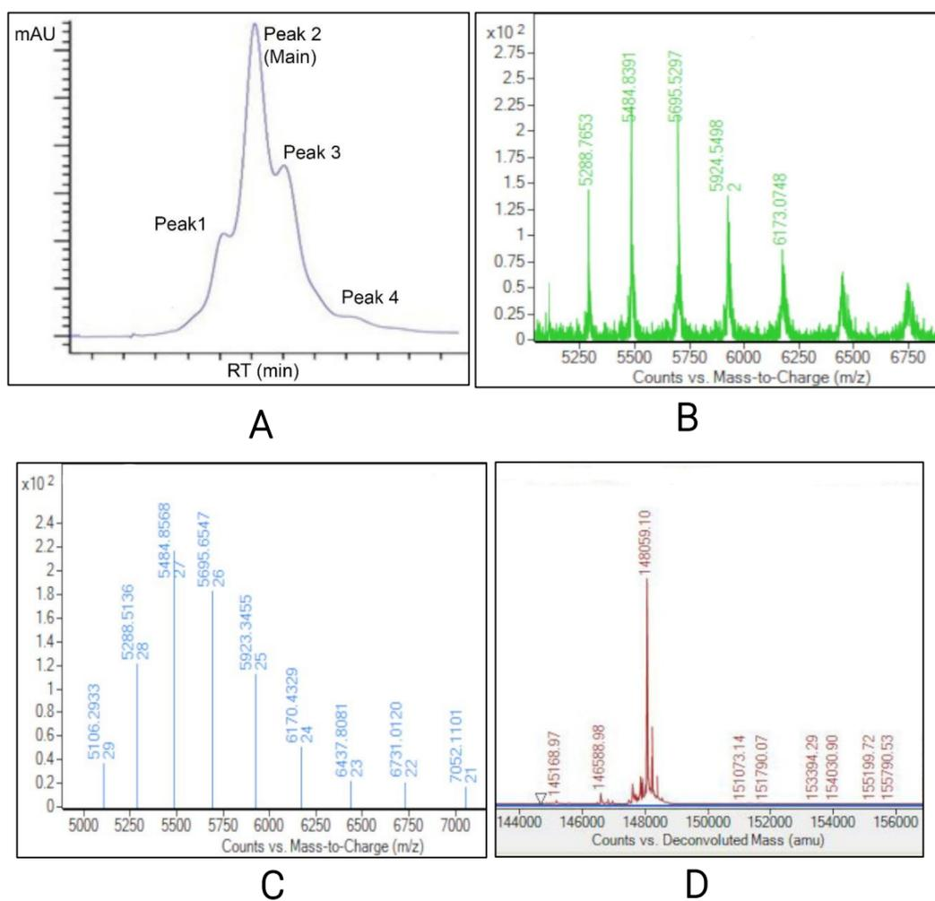
Figure 3: Native HIC-MS analysis of mAb A: (A) HIC base peak chromatogram of mAb A under the UV; (B) Charge-state pattern of mAb A which confirm ionization under native form; (C) Isotopic resolution of native mAb A; (D) Deconvoluted spectrum of mAb A.
