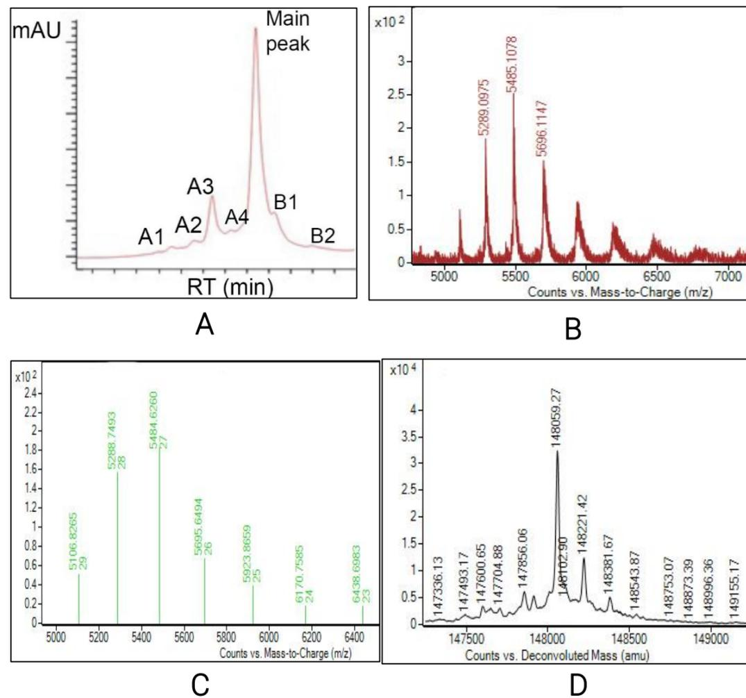
Figure 4: Native WCX-MS analysis of mAb A: (A) WCX base peak chromatogram of mAb A under the UV; (B) Charge-state pattern of mAb A which confirm ionization under native form; (C) Isotopic resolution of native mAb A; (D) Deconvoluted spectrum of mAb A.
