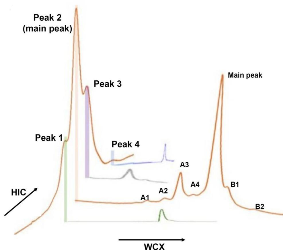
Figure 5: 2D HIC-WCX base peak chromatogram of mAb A under the UV; each HIC peak was transferred to the WCX column through a heart-cut 2D-LC method.
