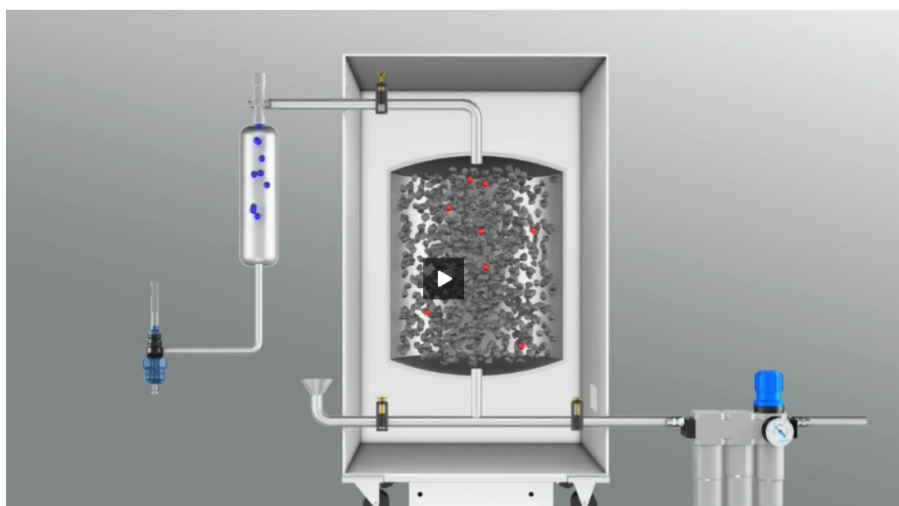
Figure 1. The nitrogen generator extracts nitrogen from compressed air to fuel the plasma.
