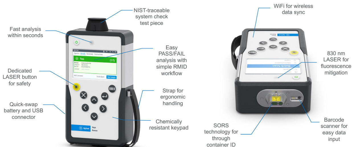
Figure 5. Key hardware features of the Agilent Vaya Raman System.
