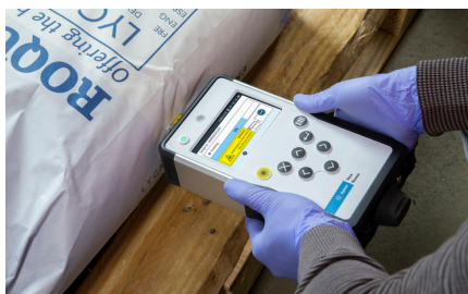
Figure 1: Using the Vaya Raman instrument to identify contents through a multilayer paper sack.
