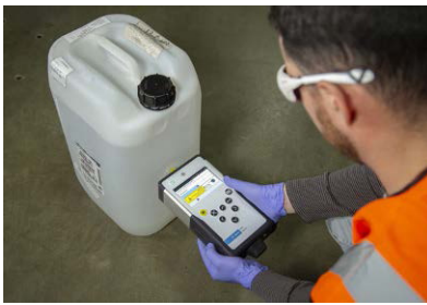
Figure 2. The Vaya verifies the identity of acetic acid in an opaque plastic container.
