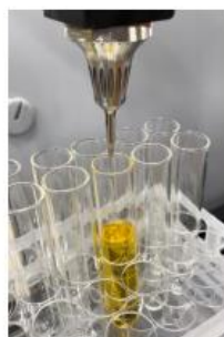
Figure 6. Fractionation to the sample vial
