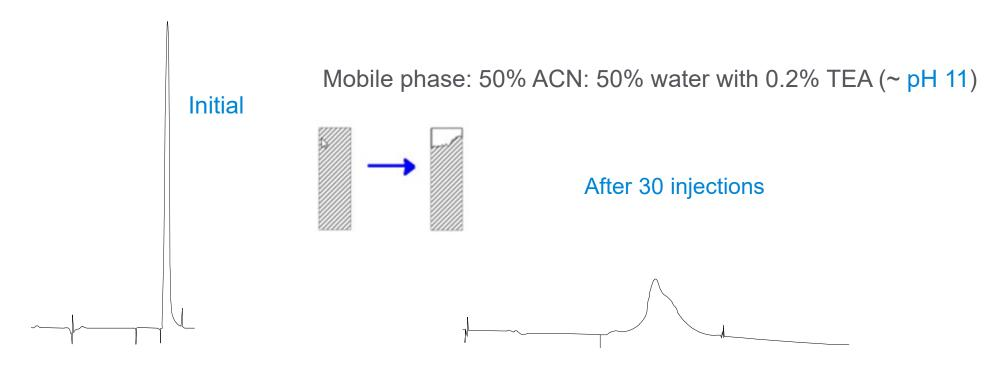
Multiple peak shape changes can be caused by the presence of a void in the column. In this case the void resulted from silica dissolved at high pH.
