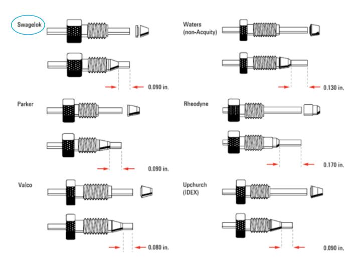
Different fitting types have different stem lengths
