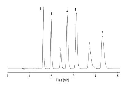
Column: ZORBAX Rapid Resolution Eclipse XDB-C8, 4.6 x 75 mm, 3.5 µm Mobile phase: 44% A: 56% methanol
