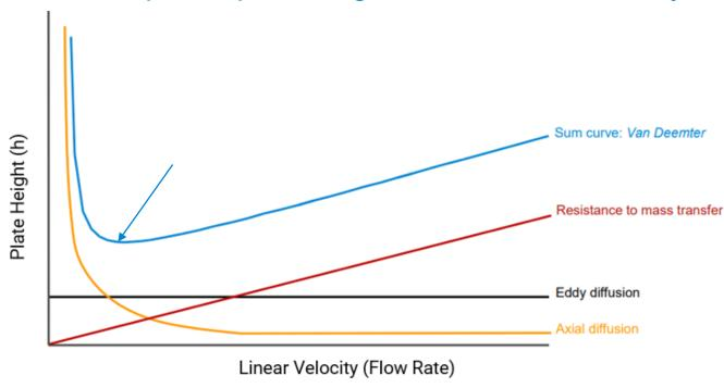
The point where minimum plate height is reached is the "optimum" linear velocity, at which the maximum plate number is reached.
