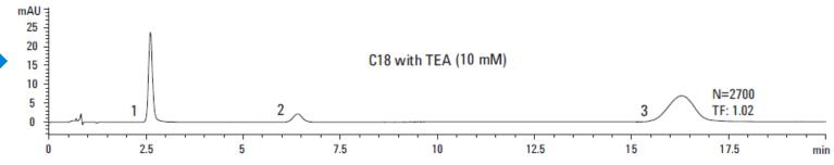
Effect of ionized acidic silanols on peak shape of amine-containing ulcer medications. A comparison of Eclipse Plus C18 and another C18 column.
