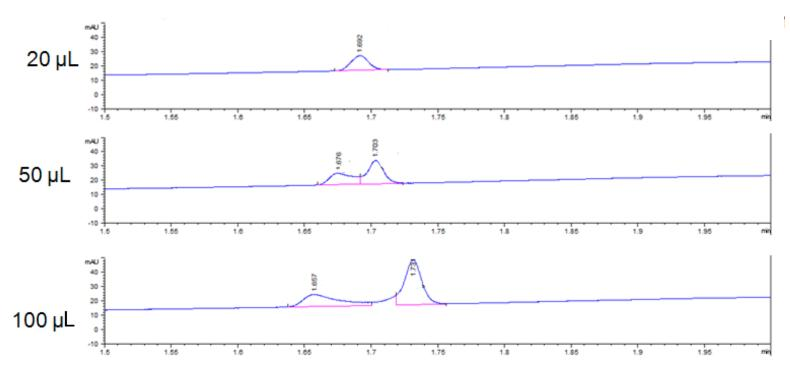
ZORBAX SB-C18, 4.6 x 50 mm, 1.8  $\mu$ m Mobile phase: 80% H<sub>2</sub>O with 0.1% TFA; 20% ACN Injection solvent; 40% H<sub>2</sub>O, 60% ACN
