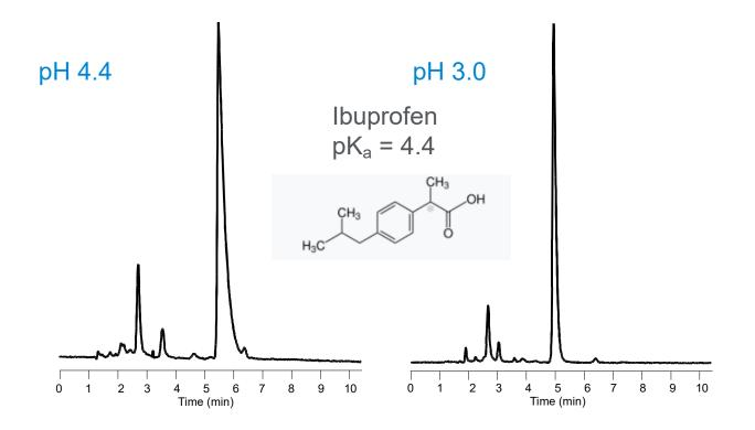
Column: ZORBAX SB-C8, 4.6 x 150 mm, 5 µm Mobile phase: 40% 5 mM KH2PO4, 60% ACN
