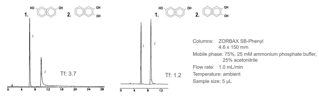
1% H<sub>3</sub>PO<sub>4</sub> in 10% acetonitrile solution is used on SB columns
