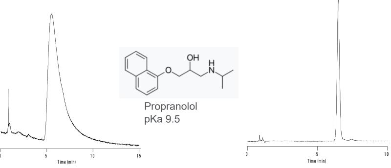
Mobile phase: 75% 50 mM KH<sub>2</sub>PO<sub>4</sub>, pH 4.4: 25% ACN flow rate: 1.5 mL/min
