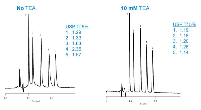
Columns: Eclipse XDB-C8, 4.6 x 150 mm, 5 µm Mobile phase: 85% 25 mM Na2HPO4 : 15% ACN pH: 7 Flow rate: 1.0 mL/min. Temperature: 35 °C Sample: Amphetamines 1. Phenylpropanolamine 2. Ephedrine 3. Amphetamine 4. Methamphetamine 5. Phenteramine
