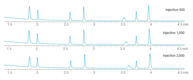
After 2,000 injections at pH 10, InfinityLab Poroshell 120 HPH-C18 showed no change in performance.
