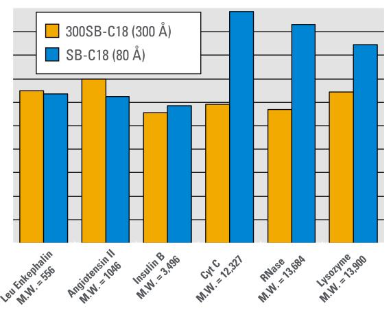
Proper pore size selection results in sharper peaks for large molecules
