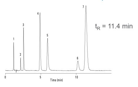
Mobile phase: 30% buffer: 70% MeOH; pH 7 buffer: 20 mM Na<sub>2</sub>HPO<sub>4</sub>; pH 11 buffer: 20 mM TEA
