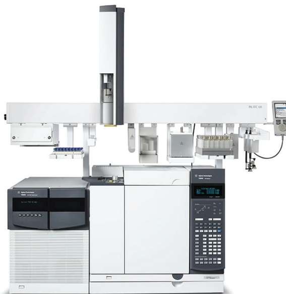
Figure 3. PAL RTC rail system combined with an Agilent 7890B GC + 5977B High GC/MSD.
