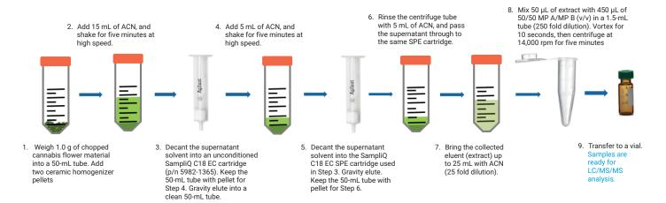
Figure 1. Schematic representation of sample preparation procedure for LC/MS/MS analysis.
