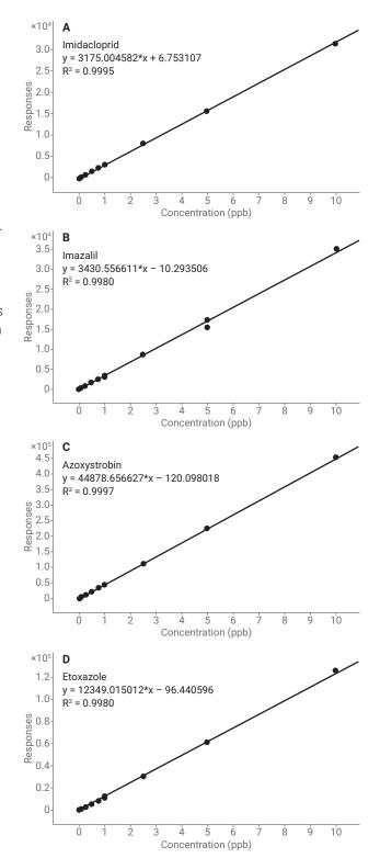
**Figure 5.** Select Ultivo LC/MS/MS calibration curves. A) Imidacloprid, B) Imazalil, C) Azoxystrobin, D) Etoxazole.
