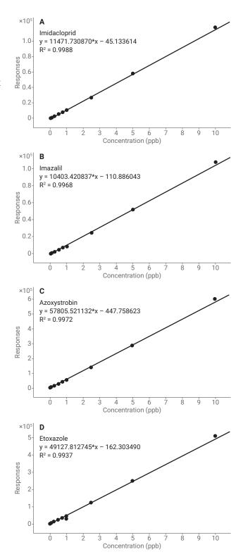
**Figure 3.** Select 6470 LC/MS/MS calibration curves. A) Imidacloprid, B) Imazalil, C) Azoxystrobin, D) Etoxazole.
