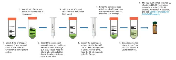
Figure 2. Schematic representation of sample preparation procedure for GC/MS/MS analysis.
