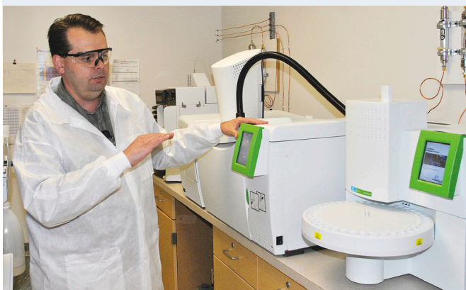
Mark Thomas, a Chemist with Weld County's Department of Public Health and Environment, running the Clarus GC mass spectrometer
