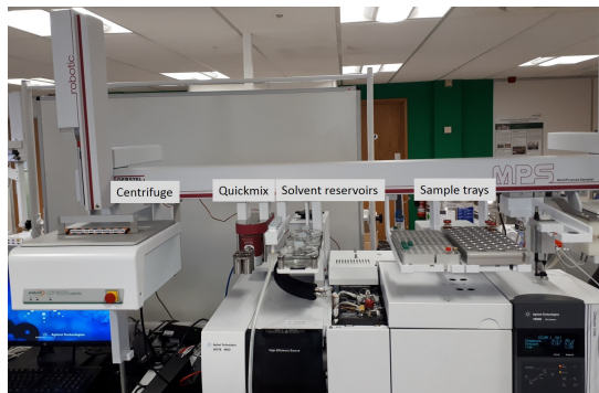
Figure 1: GERSTEL Dual Head Robotic MPS on top of Agilent GC7890 B coupled to 5977 B MS (HES)
