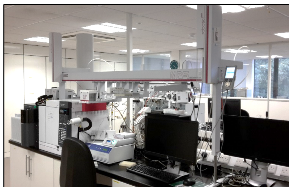
Figure 2: MPS Robotic Dual Head equipped with DHS and mounted onto Agilent 7200 GC-QTOF
