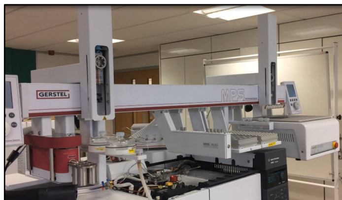
Figure 1: GERSTEL MPS equipped with Automated Liner Exchange (ALEX) for LVI method optimisation
