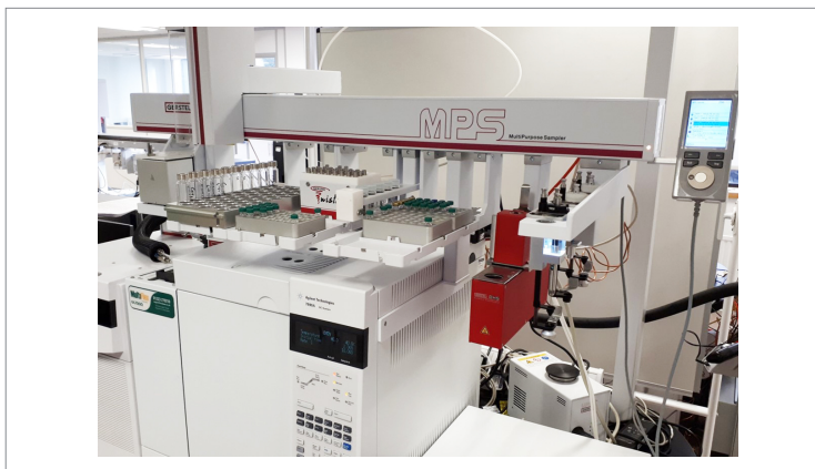
Figure 1: MPS Robotic Pro (tool exchange) and DHS on Agilent GC-MS
