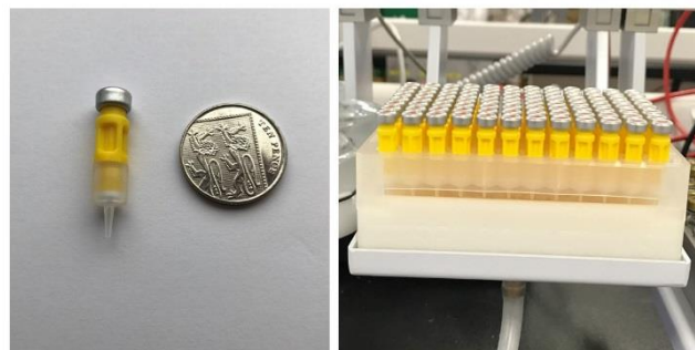
Figure 1: Instrument Top Sample Prep (ITSP) miniaturised cartridges for smart SPE and 96 well plate format ITSP tray.
