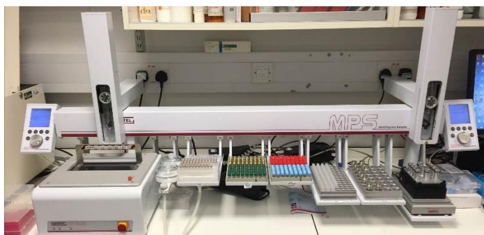
Figure 2: GERSTEL Dual Head MPS for the extraction and derivatisation of amino acids for GC-MS analysis
