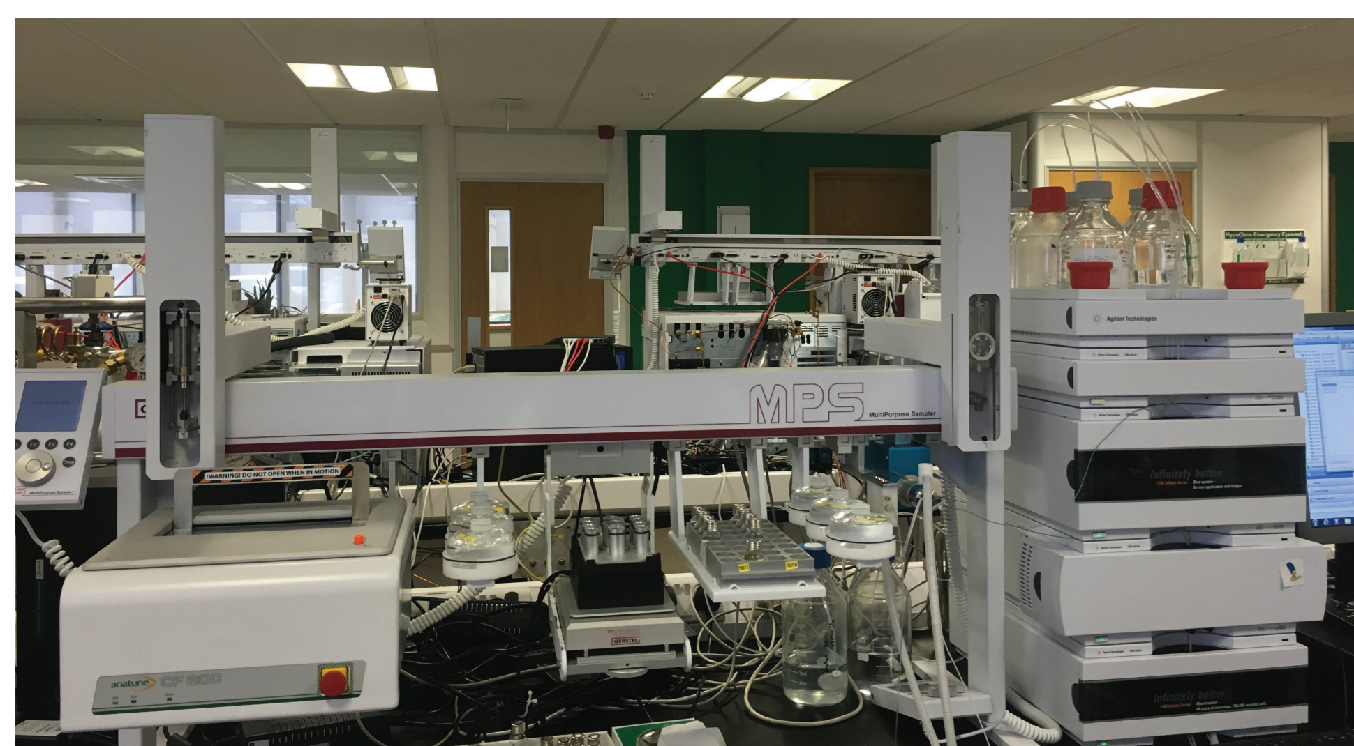
Figure 2 GERSTEL Dual Head, mVortex and centrifuge with Agilent LC 1260 with Diode Array detection at Anatune
