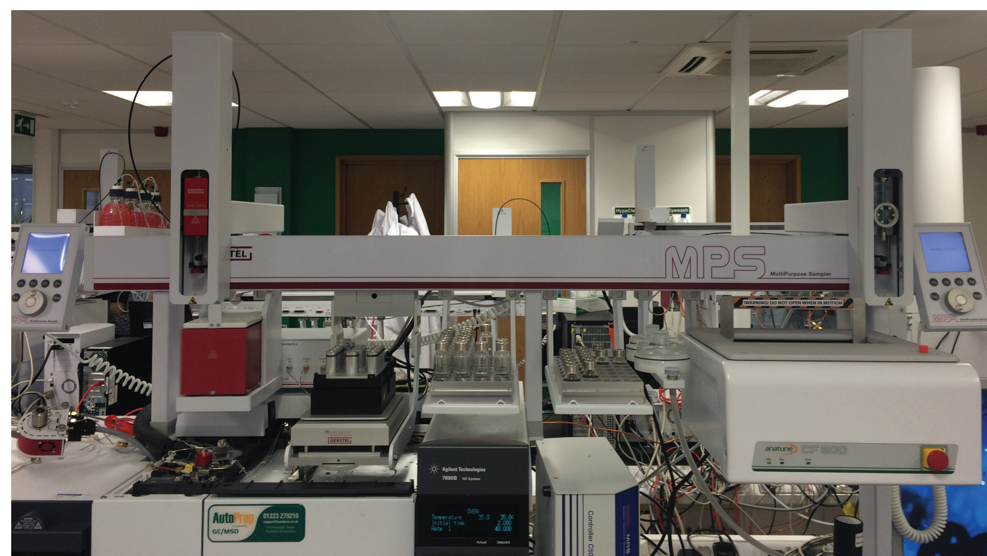
Figure 1 GERSTEL Dual Head, mVortex (automated vortexer) and centrifuge with Agilent GC-MS (5977) at Anatune
