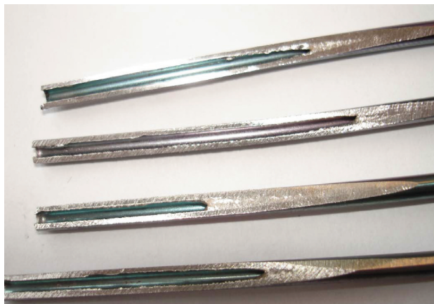
1/8 inch tubing with internal Agilent UltiMetal Plus treatment
