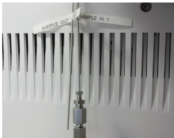
Figure 1. Examples of 1/16 inch stainless steel transfer lines in the flow path. For the analysis of (re)active components these should be deactivated.
