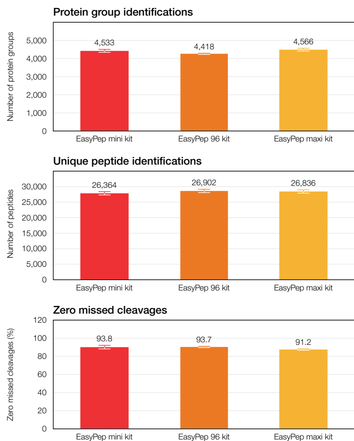
Figure 3. Comparison of the EasyPep Mini, 96, and Maxi MS Sample Prep Kits for processing HeLa cell lysates. All three formats provide comparable peptide and protein identifications with high digestion efficiency (percentage of zero missed cleavages with high reproducibility).
