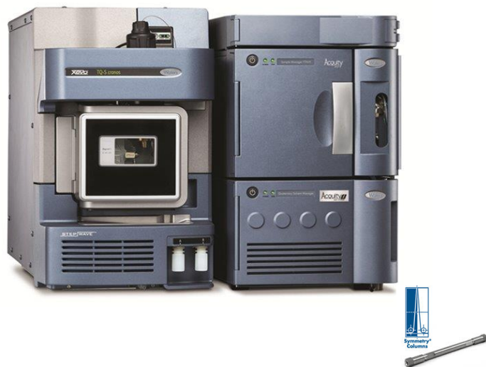
Figure 2: Xevo TQ S Cronos with Acquity UPLC H-Class Plus , and Symmetry C8 Column
