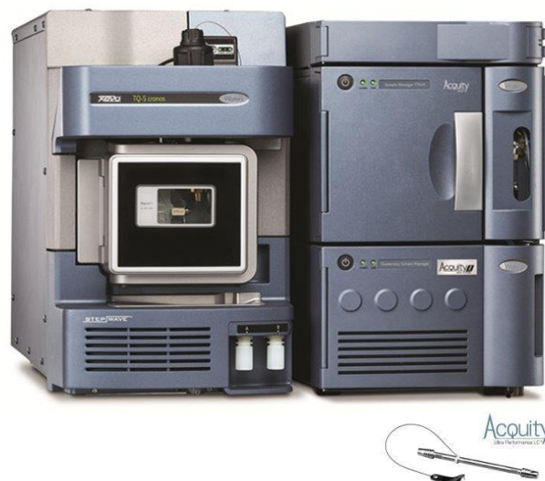
Figure 3: Xevo TQ S Cronos with Acquity UPLC H-Class Plus, and Acquity UPLC BEH C18 Column
