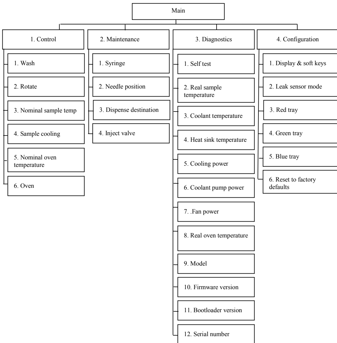
Fig. 35: Autosampler menus (here ACC-3000T)
