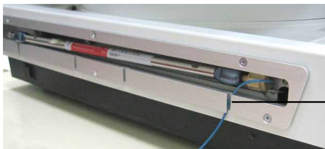
Fig. 15: Column in column chamber
