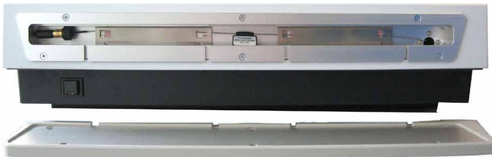
Fig. 14: View into the column chamber
