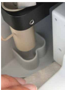
Fig. 40: Drying the leak sensor
