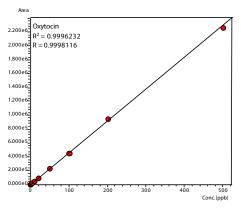
Fig. 3 Calibration Curve of Oxytocin (0.1 to 500 ng/mL)
