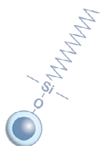
Fig. 2 Representation of the Shim-pack Velox C18 Stationary Phase
