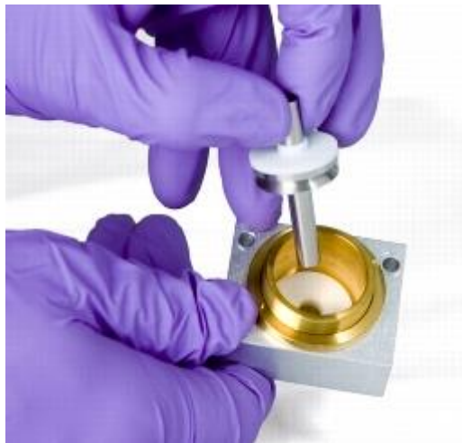
Remove the collector and Upper/lower PTFE Insulators
