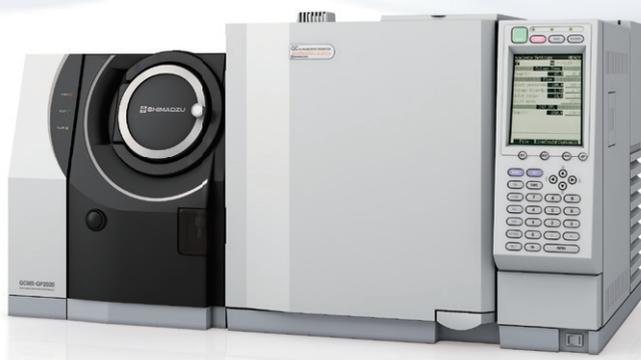
The combination of the GCMS-QP2020 single quadrupole mass spectrometer with the FID-2010 Plus detector allows a very simple and robust determination of nicotine concentration (by flame ionization), identification of CAS# and IUPAC-name (by mass spectrometry), and quantitation of many flavor compounds in e-liquids.
