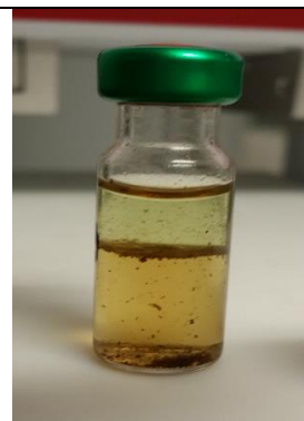
Figure 2: Extraction mixture with the FAME's in the top hexane layer
