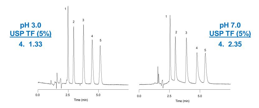
Tip: Reducing mobile phase pH reduces interactions with silanols and peak tailing.
