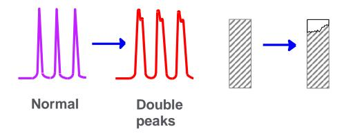
Tip: A similar effect can be caused by partially plugged frit.
