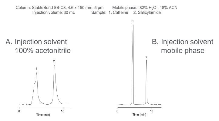
Tip: Injecting in a solvent stronger than the mobile phase can cause peak shape problems, such as peak splitting or broadening.
