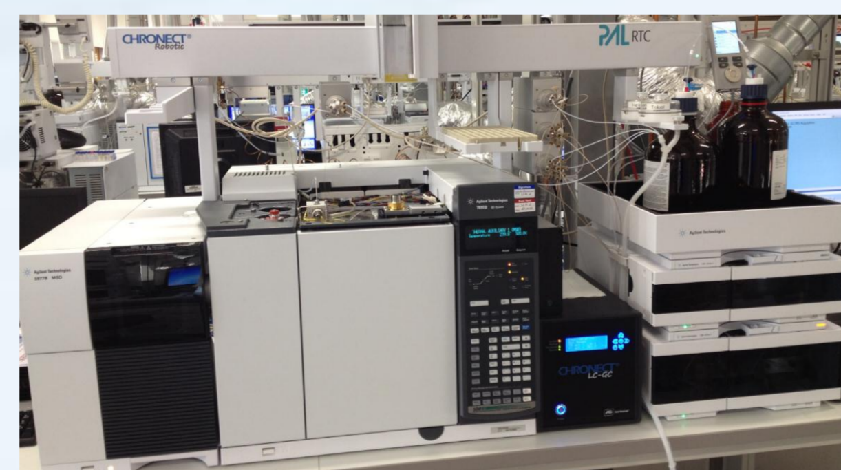
Figure 3 LC-LC-GC-MS system by Axel Semrau
