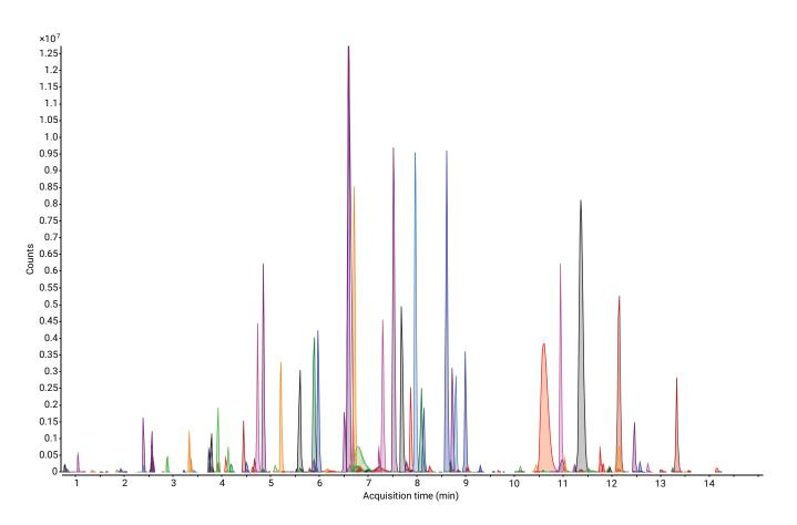
Figure 2. ECC of peptides from Trypsin/Lys-C digested NISTmAb standard RM 8671, separated using an Agilent AdvanceBio Peptide Mapping column.
