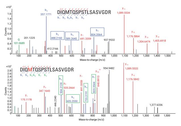
**Figure 5.** Post-translational modification (methionine oxidation) analysis. MS/MS spectrum of native and Met-oxidized peptides (light chain peptide 1-18). Top: native peptide, Bottom: oxidation at Met 4 (confirmed fragment ions in green boxes).
