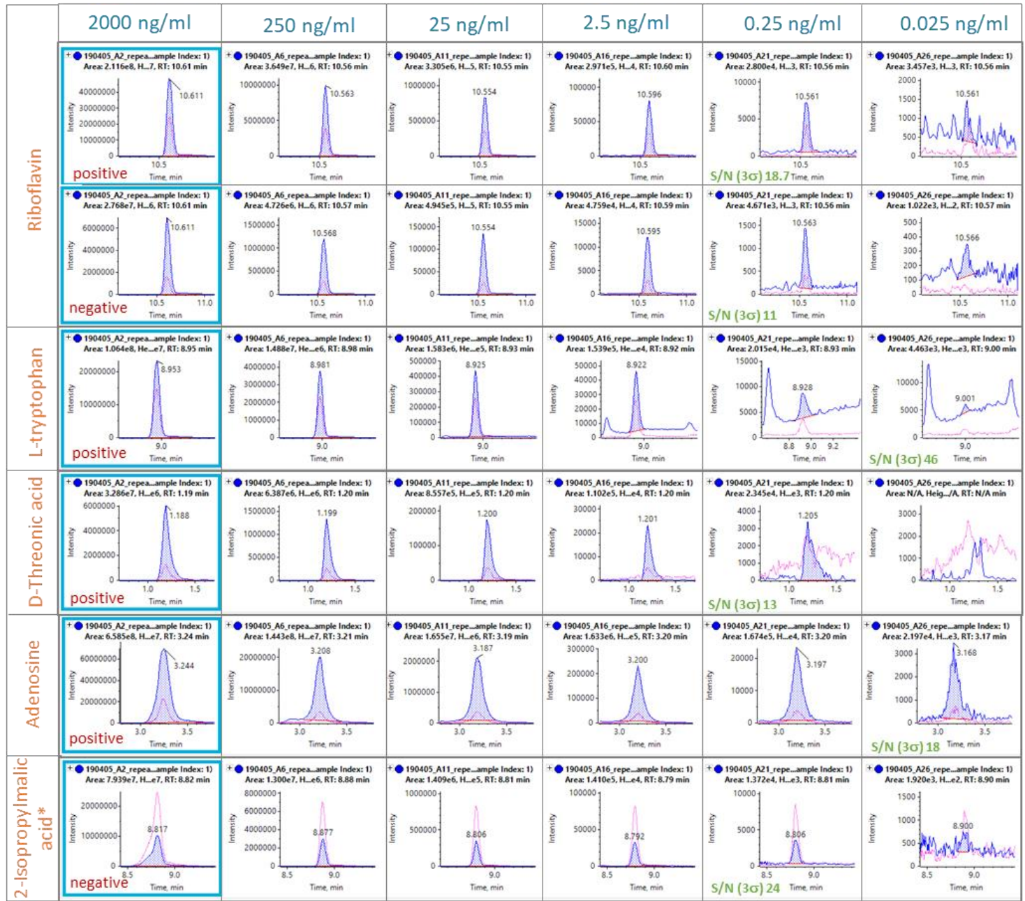
Figure 8. Extracted Ion Chromatograms shows two MRMs per selected compound from cell culture group class. In the cell culture standard mixture the LDR vary from 2- to 6-orders of magnitude depending. Blue XIC is MRM and pink XIC is MRM2 for selected compound. The Signal to Noise ratio values indicating the LLOQ of compound. * 2x higher load on a column.
