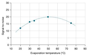
Figure 3. Influence of the evaporation temperature on the signal-tonoise ratio of a 0.1% topiramate solution with an optimum value at 50 °C (see References 5 and 6 for more details)
