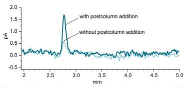
Figure 5. Influence of post-column addition with isocratic flow of ACN (0 vs 1 mL/min) on the response of impurity A
