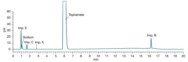
Figure 4. Impurity spiked solution of topiramate measured by means of the current related substances test for topiramate of the Ph. Eur. on the Vanquish Flex UHPLC system
