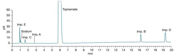
Figure 6. Chromatogram of an impurity spiked test solution of topiramate performed on the Vanquish Flex UHPLC system; gradient conditions: 0–5 min 20% B; 5–15 min 20→50% B; 15–20 min 50% B; 20–20.1 min 50→ 20% B; 20.1–25 min 20% B
