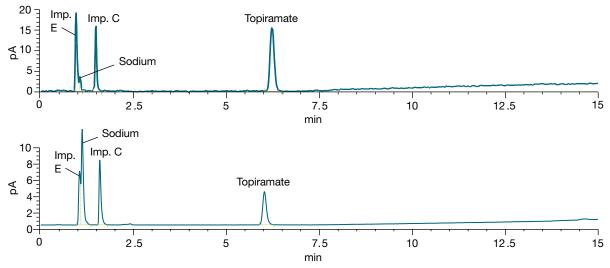
Figure 2. Comparison of the chromatograms obtained with two different topiramate reference solutions measured with different laboratory instrumentation at different times (c). Top: Vanquish Flex UHPLC system; bottom: legacy HPLC system.
