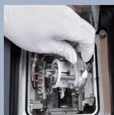
Re-engineered ion guide improves robustness without compromising on sensitivity. Maintenance of UF-Qarray II and UF-Lens II can be performed easily without tools.
