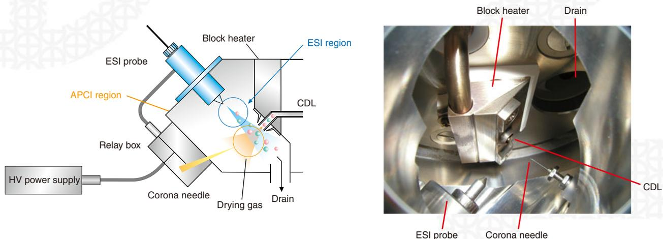
Fig. 5: Duis-2010 Structural Diagram and Photo of Interior
