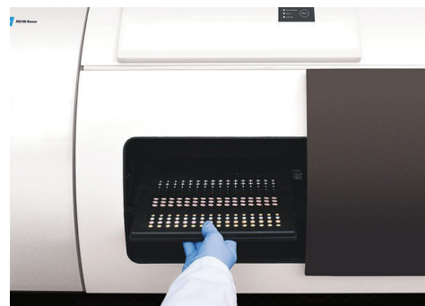
2. Place the tray in the instrument for analysis. No sample preparation is required.
