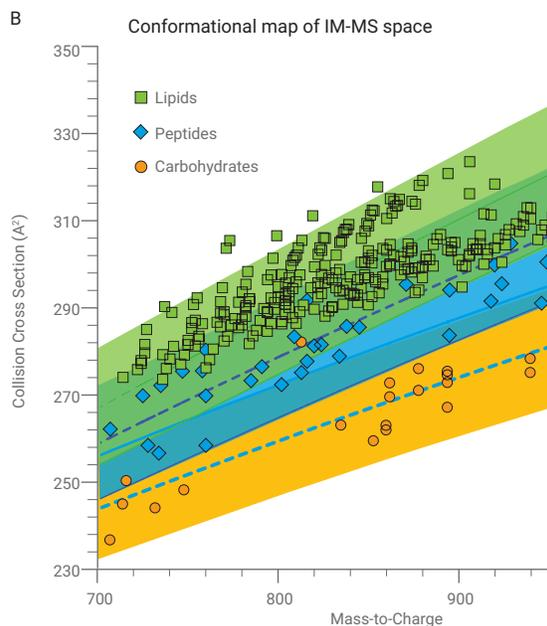
B) A zoomed-in region with a high signal density. Distinguishing individual ion signals by the  $m/z$  measurement alone is challenging. Yet, the combined structural separation of IM Q-TOF allows the data to be delineated into chemical class-specific regions.\*
