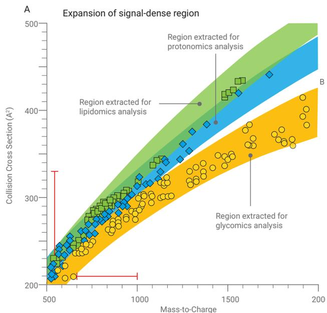
A) A sample containing lipids, peptides, and carbohydrates was infused directly into the instrument, then resolved using 2-D IM Q-TOF analysis by collision cross section and  $m/z$ . Conformational space maps allow complex mixtures to be separated based on different biomolecular classes with little front-end sample workup.\*
