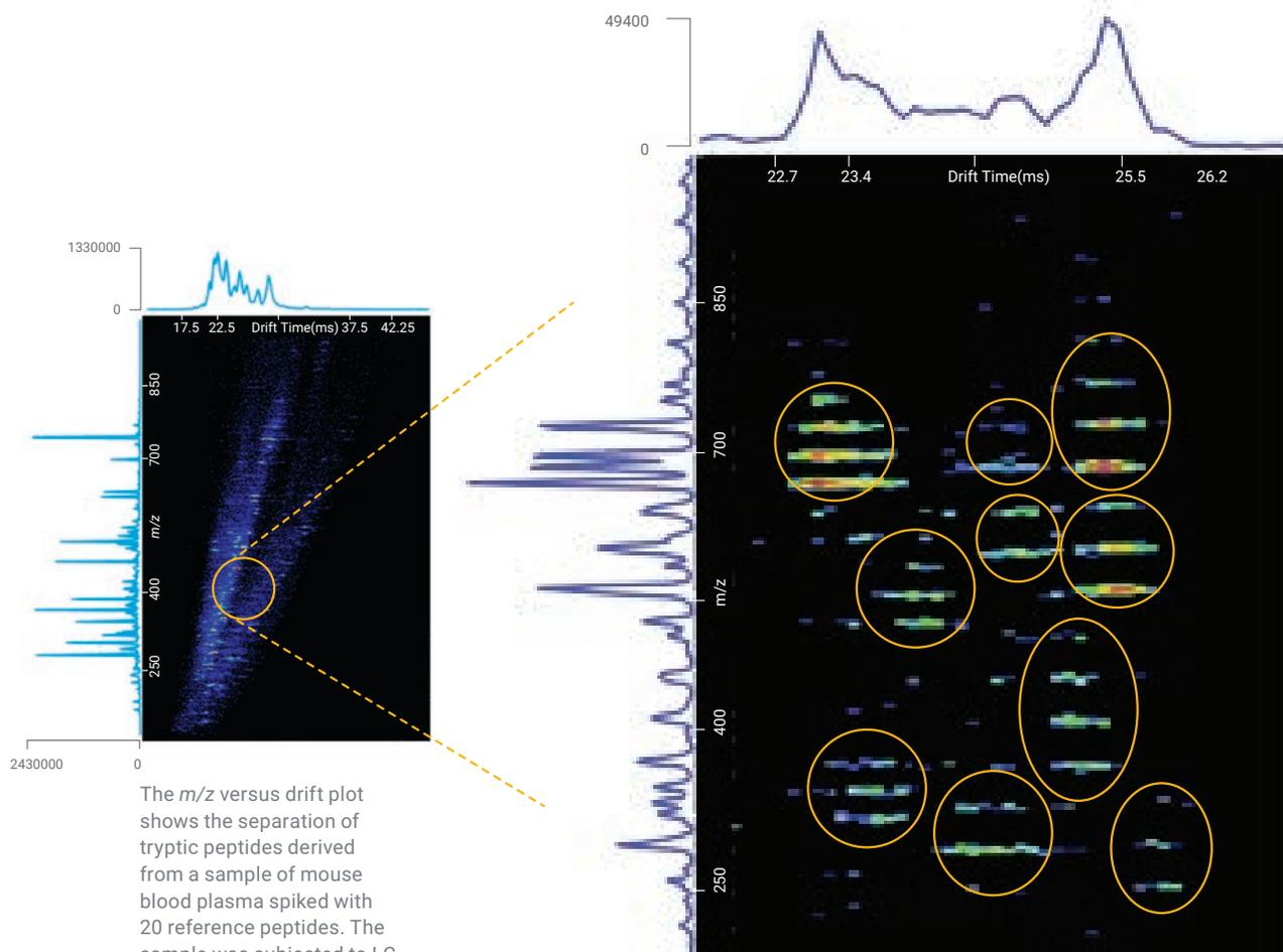
The  $m/z$  versus drift plot shows the separation of tryptic peptides derived from a sample of mouse blood plasma spiked with 20 reference peptides. The sample was subjected to LC separation for 15 minutes before IM Q-TOF analysis.
