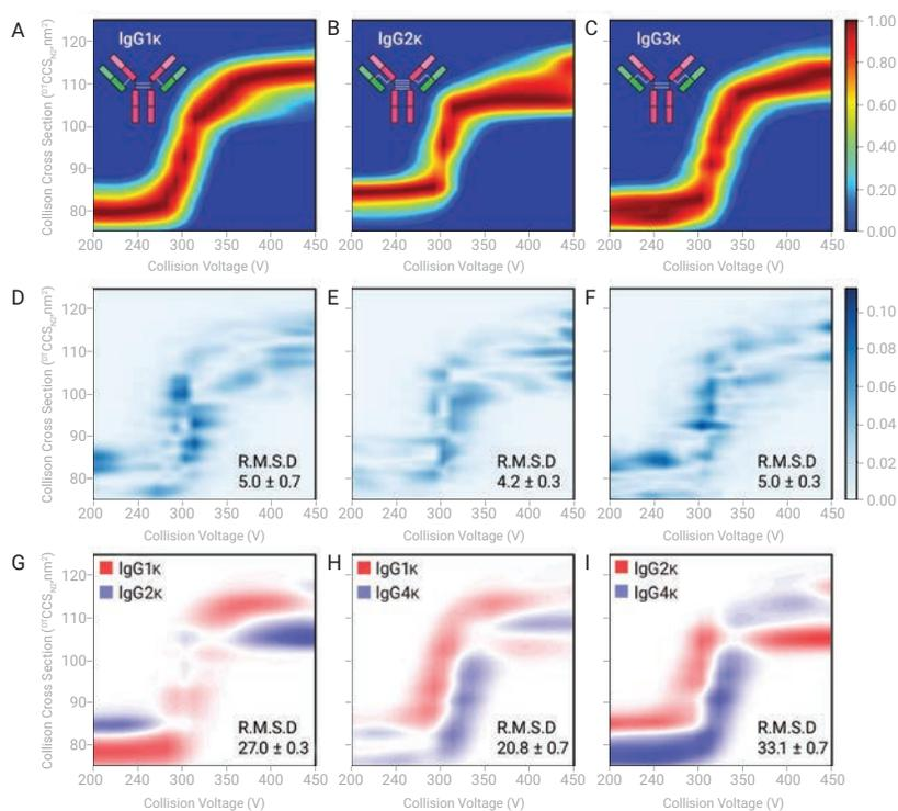
Results from CIU experiments. Figures A–C: CIU curve for IgG1 kappa, IgG2 kappa and IgG3 kappa. Figures D–F: CIU curve average Root Square Mean Deviation (RMSD) value for multiple replicate runs of IgG1–3 kappa. Figures G–I: Comparison CIU curve average RMSD value for IgG1 kappa versus IgG2–4 kappa, with the image showing the comparison plots for the summed IgG's kappa.
