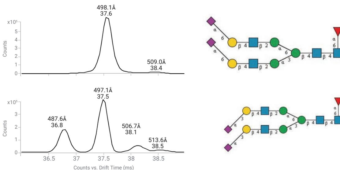
Differentiation of isomeric *N*-glycans by their HR conformer distribution fingerprint and CCS values. The *N*-glycans were derivatized with 2-aminobenzoic acid at the reducing end and measured in negative ion mode as  $[M-2H]2-$  ions.
