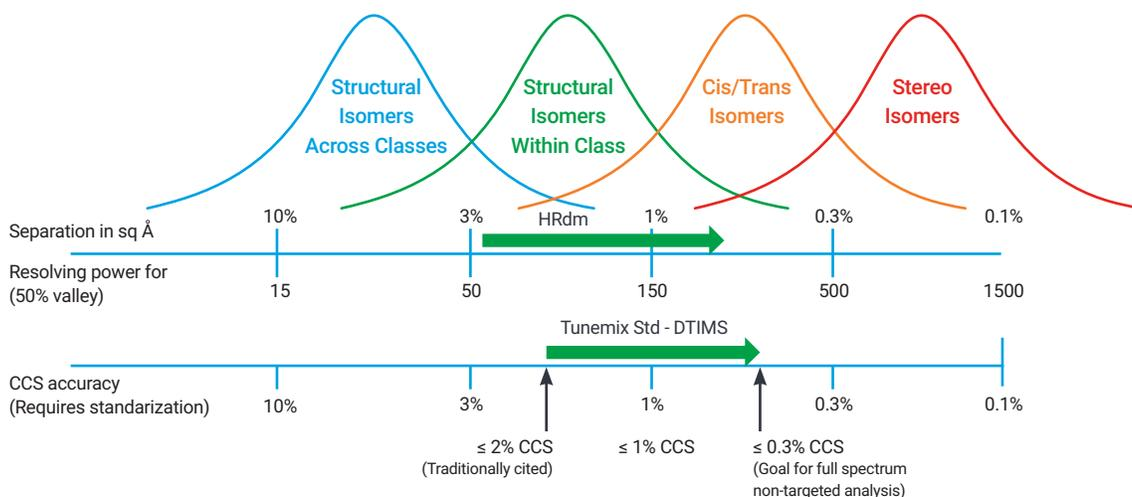
Different types of isomers require increasing IM resolving power. The same applies to identification, where CCS accuracy is of critical importance.
