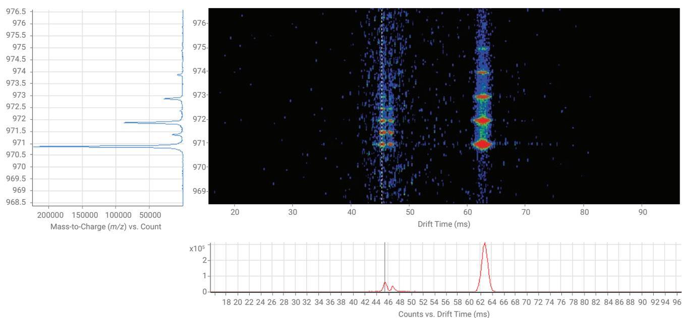
Both positive ion and negative ion nitrogen drift data of the same compound (cyclodextrin) in protonated and deprotonated form. CCS calculations in positive and negative mode showed CCS values within 2% accuracy. A) One well resolved drift peak in positive mode. B) Two different peaks (singly charged monomer as well as doubly charged dimer) in negative mode. Lower intensity peak contains two different conformers, possibly indicating that the dimers exist as two conformers.
