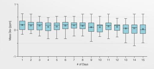
Through the use of Thermo Scientific EASY-IC ion source, sub-ppm mass accuracy is consistently delivered without user intervention for at least five days. A panel of veterinary drugs with *m/z* range from 160...900 was analyzed at 100  $\mu$ g/L over a 15 day period with continual polarity switching, providing exceptional mass accuracy.
