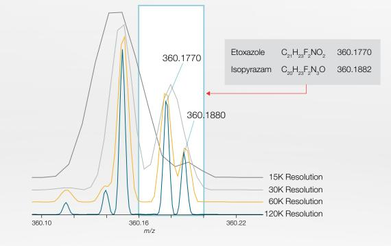
Full-scan mass spectrum of etoxazole and isopyrazam, measured using the Orbitrap Exploris 120 mass spectrometer at a resolution (R) setting up to 120,000 (FWHM) at *m/z* 200, demonstrates outstanding resolving power.
