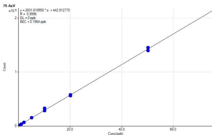
**Figure 4.** Calibration curve for iAs (represented by As(V)).
