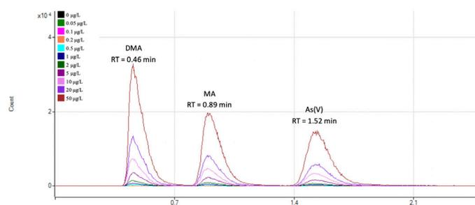
**Figure 2.** Overlaid chromatograms of calibration standards between 0.05 and 50 μg/L prepared in the mobile phase.
